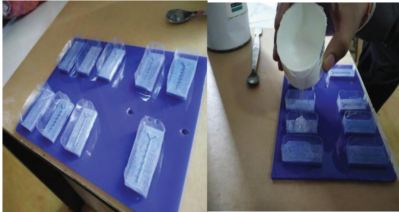
Fig. 7 Pouring of PDMS into Mold cavity
